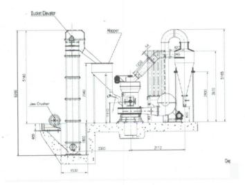
Figure 2. The proposed layout of YGM75 Milling plant
